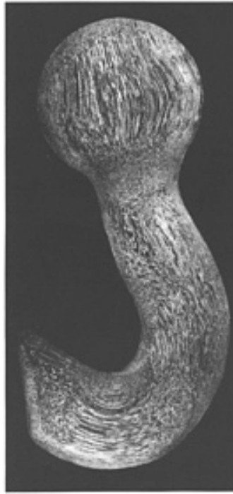
Fig. 4 Flow lines, as shown in a longitudinal section taken through a hook that was forged from 4140 steel
