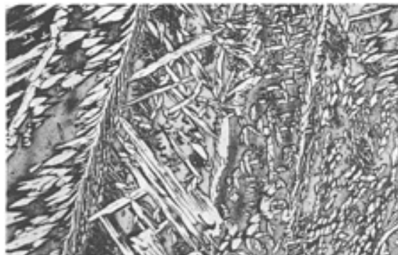
Fig. 44 Photomicrograph of a duplex stainless weld obtained using consumables with increased nickel to retain sufficient austenite in the weld. Typical weld metal microstructure for gas metal arc weld in 19.1 mm (0.752 in.) thick plate. The light-etching phase is austenite. The micrograph shows a cross section etched in Groesbeck's reagent. 200×
