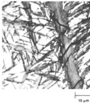
Fig. 17 Light micrograph of plate martensite and retained austenite in an Fe-1.39C alloy. Source: Ref 25
