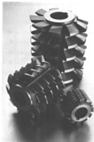
Fig. 16 Gear hobs made from P/M high-speed tool steels. Courtesy of Speedsteel Inc.
