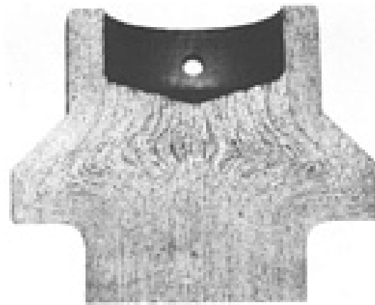
Fig. 10 Uniform, unbroken grain flow around the contours of the forged head of a threaded fastener. The uniform, unbroken grain flow minimizes stress raisers and unfavorable shear planes and therefore improves fatigue strength.
