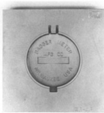
Fig. 25 P/M H19 die produced using prealloyed powder and the ceramic core process. Courtesy of Crucible Materials Corporation
