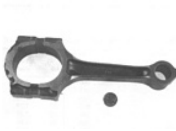
Fig. 21 Powder forged connecting rod for 1.9 L automobile engine. A similar rod will be used in the modular engine.
