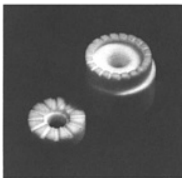
Fig. 21 Multiple-crevice cylinders for use in crevice corrosion testing. Source: Ref 59
