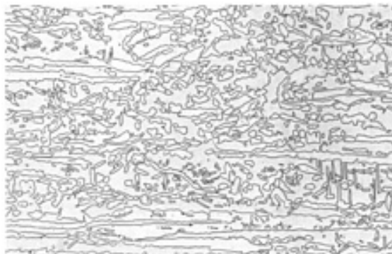
Fig. 43 Photomicrograph of a duplex stainless steel showing elongated austenite islands in the ferrite matrix. The mill-annealed 19.1 mm (0.752 in.) thick plate sample is a longitudinal section etched using 15 ml HCl in
