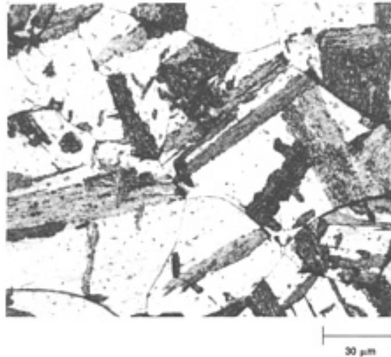
Fig. 5 Light micrograph showing patches of upper bainite (dark) formed in 4150 steel partially transformed at 460 °C (860 °F). Courtesy of F.A. Jacobs
