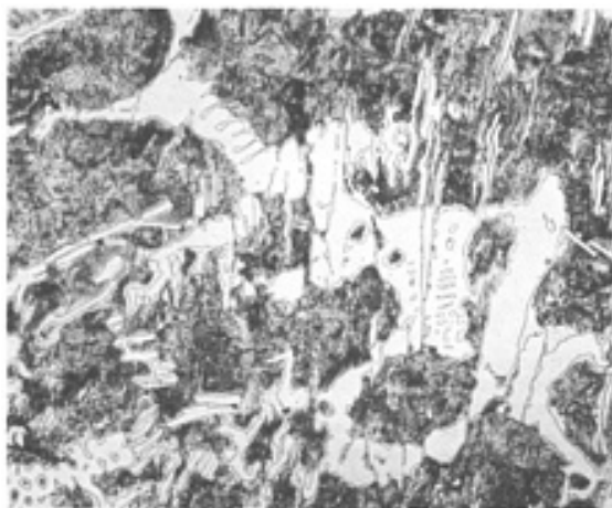
Fig. 1 Structure of as-cast malleable white iron showing a mixture of pearlite and eutectic carbides. 400×
