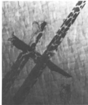
Fig. 19 Inhomogeneous deformation in CMSX-2 ( T_1 heat treatment) during primary creep at 760 °C (1400 °F). Source: Ref 29
