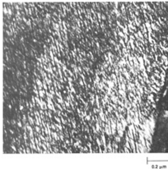
Fig. 19 Transmission electron micrograph showing effects of transition carbide precipitation (dark contrast) in fine structure of a plate of martensite in an Fe-1.22C alloy tempered at 150 °C (300 °F). Source: Ref 29
