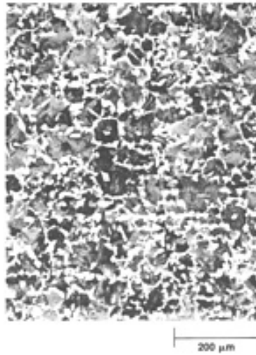
Fig. 14 Grain structure of a microalloyed steel bar product of composition Fe-0.38C-1.18Mn-0.16V-0.018N. Source: Ref 21
