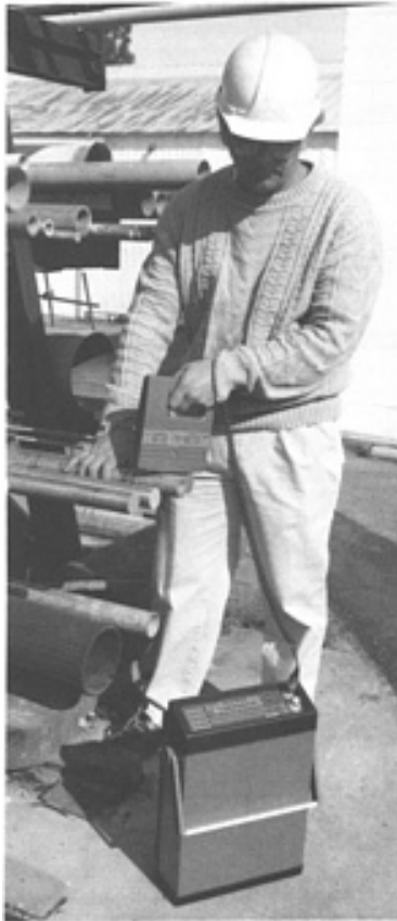
Fig. 8 Portable x-ray spectroscope. Source: Ref 7
